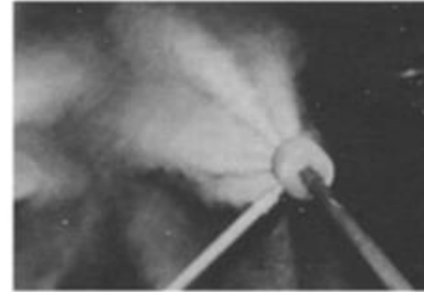
Atomised scrubbing spray nozzles
